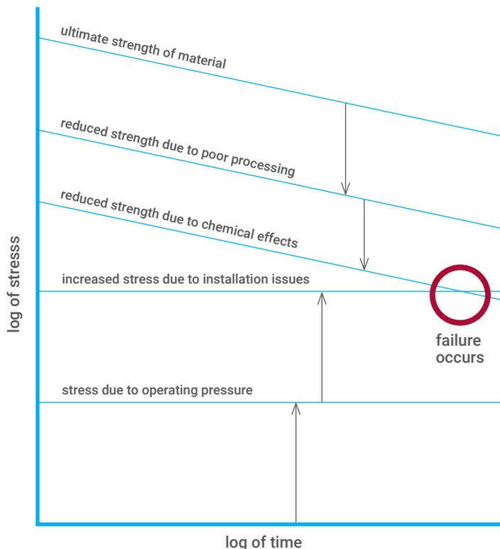
On the other hand, if mechanical stresses are low, and/or the processing of the material has been sufficient to achieve good molecular entanglement, then the plastic material may perform for a long time with no ill effects, even though it has been used in direct contact with a chemical classified as “incompatible.”
